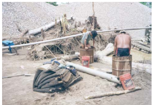
Gold remains in the carpets, which are placed in the bottom of the sluices/washing tables. The carpets are tread on in the barrels and the remaining sand is panned by the gold pan with mercury (Photo: Kauko Launonen)
