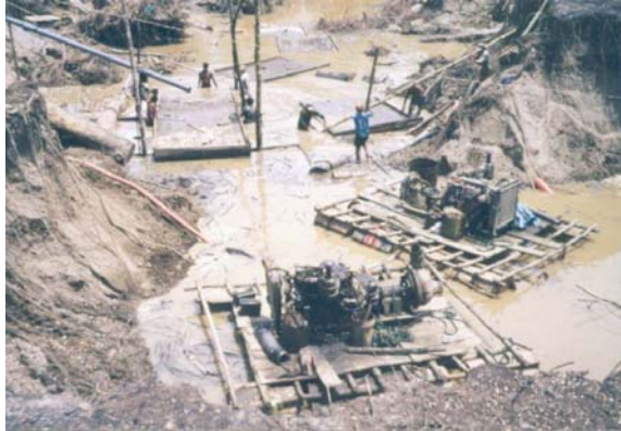
In the front there are machines, which suck the sludge from the bottom of the pit. Behind the men are preparing to lift the washing tables/sluices up to the poles. They are lifted as high as possible so that they don't have to move them continuously when the heap of tailings grows (Photo: Kauko Launonen)
