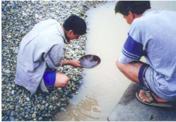
Peruvian gold pan is a round-bottom. The gold is very fine and mercury is commonly used (Photo: Kauko Launonen)
