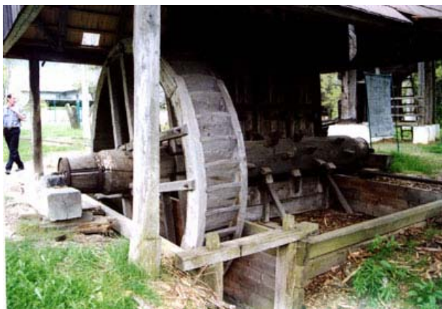
Open-air museum in Rosia Montana plant. The water driven wood stamps crushed the ore prior to gravitation treatment.
