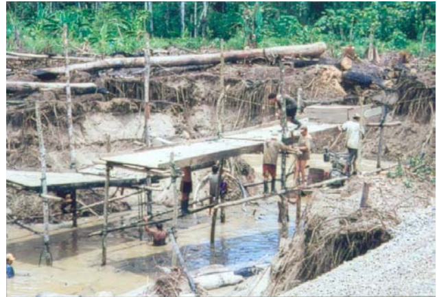
The washing tables/sluices are lifted up to the poles with help of ropes and the coarse carpets are spread on the tables (Photo: Kauko Launonen)
