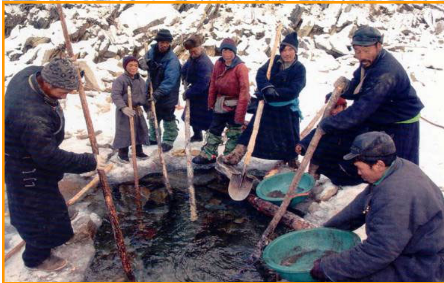
Digging up the mud, then slowly sifting. And finding 5 to 10 grams of gold in a day. This is the classical hard work for gold panners.
